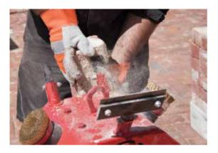
TWO OPERATORS CAN CLEAN IN EXCESS OF 2000 BRICKS PER DAY
